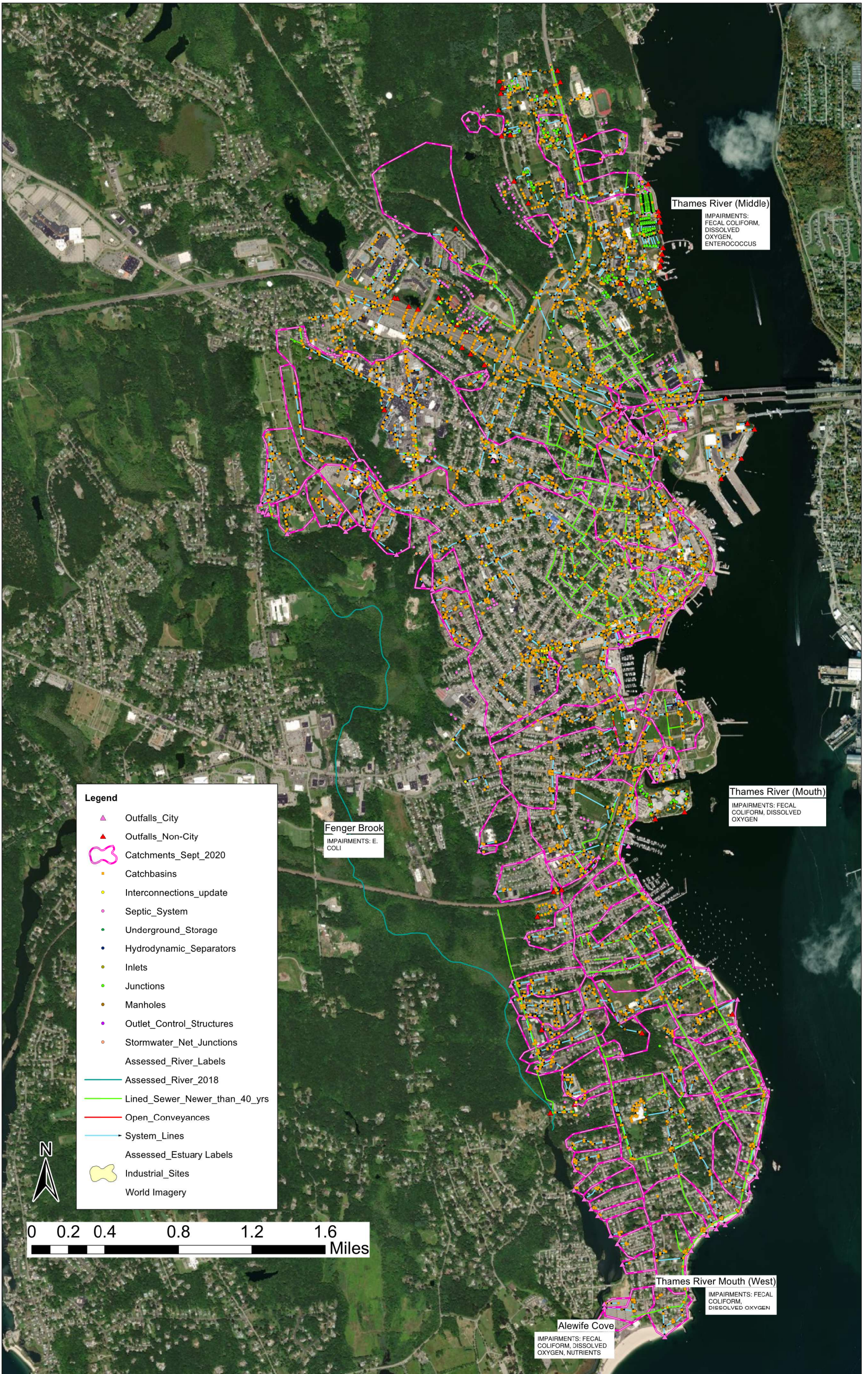
NEW LONDON STORM SEWER SYSTEM MAP
